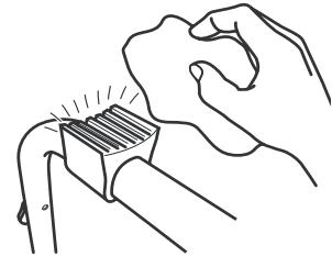
**GB.** Refer to the enclosed application list to find the correct position for the extendable feet X, Y or Z. Insert the bolts from the outside faces, fit the thumb screw nuts to the inside of the carrier frame. Before offering the carrier to your vehicle ensure the rear window/bodywork and the rubber feet on the vehicle support arm are clean and free of dust.
