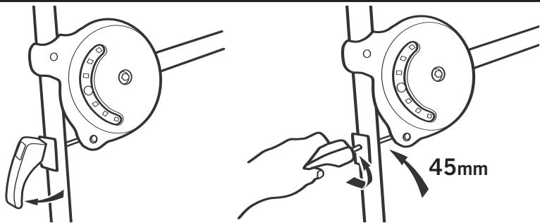
**GB.** Release the two carrier clamping levers and turn the handles anti-clockwise until the angle adjusters are fully opened, exposing approximately 45mm of the bolt.
