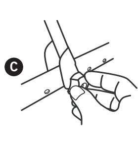
**GB.** Refer to the enclosed application list to find the correct clamp bolt hole for your car. Insert the bolts, from the outer faces, through the metal clamps and the vehicle support arm. Fit the thumb screw nuts on the inside of the vehicle support arm.
