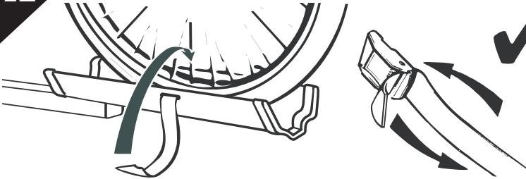
**GB.** Feed the wheel straps through the wheel and into the cam buckle. **WARNING:** ENSURE THAT THE STRAPS ARE INSERTED THROUGH THE CAMBUCKLES IN THE CORRECT DIRECTION.
