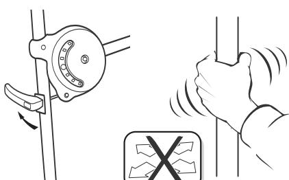
**GB.** Once you have set up the carrier for your first use all adjustments can remain in position. When re-fitting release the two clamping levers (as step 2) offer the carrier to the vehicle (as in step 10) fitting the carrier feet to your tailgate 1st and then the metal fitting kit clamps 2nd. Repeat step 8 until firmly fixed in all directions.
