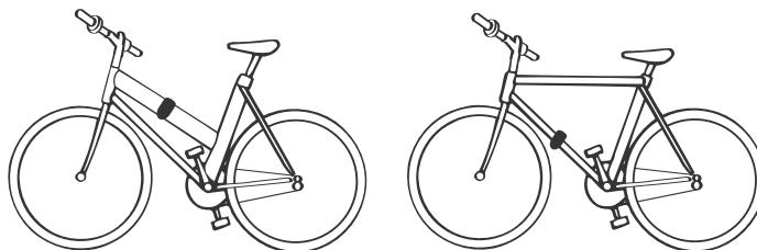
**GB.** The cycle frame locators can be adjusted to best suit the angle of ladies' and childrens' etc cycle frames. **IMPORTANT:** Do not open your boot/tailgate with the cycle carrier in position.
