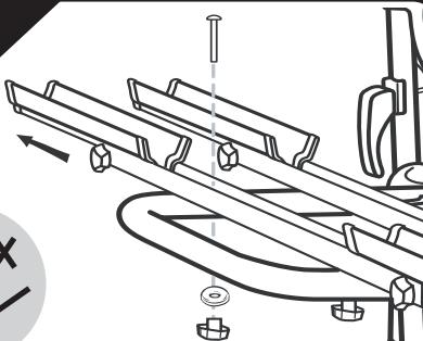
**GB.** Extend the cycle 'V'-channels in a telescopic motion to expose the holes in the cross frames. Mount the cycle support frame with the bolts and plastic nuts provided.
