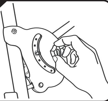
**GB.** Fit the thumb screw nuts to the inside face of the angle adjusters.
