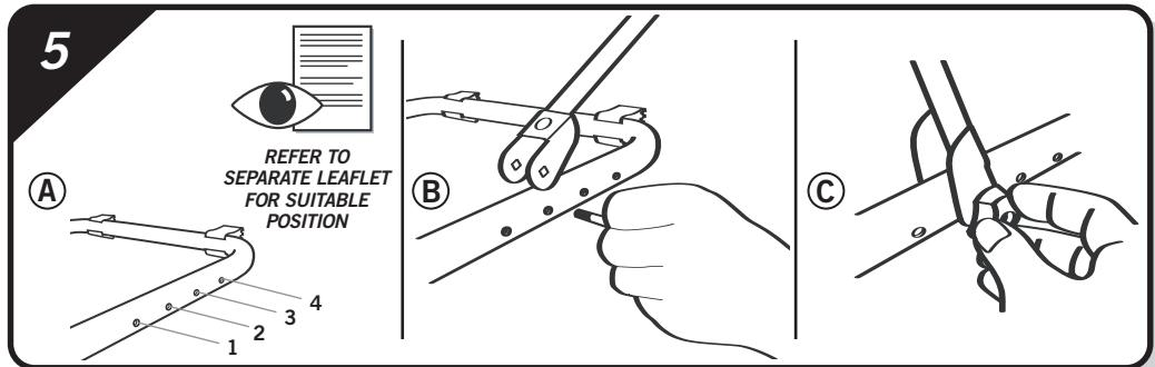
**gb.** Refer to the enclosed application list to find the correct clamp bolt hole for your car. Insert the bolts, from the outer faces, through the metal clamps and the vehicle support arm. Fit the thumb screw nuts on the inside of the vehicle support arm.
