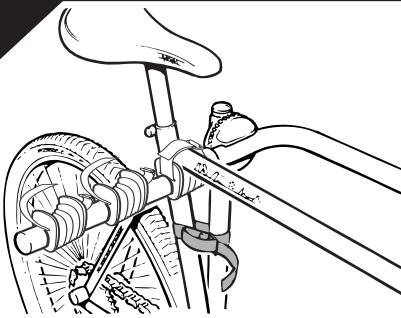
**GB. IMPORTANT:** Using the fitted RED webbing straps, secure the first cycle to the carrier main frame. Failure to use these straps will result in the cycles falling off the carrier.
