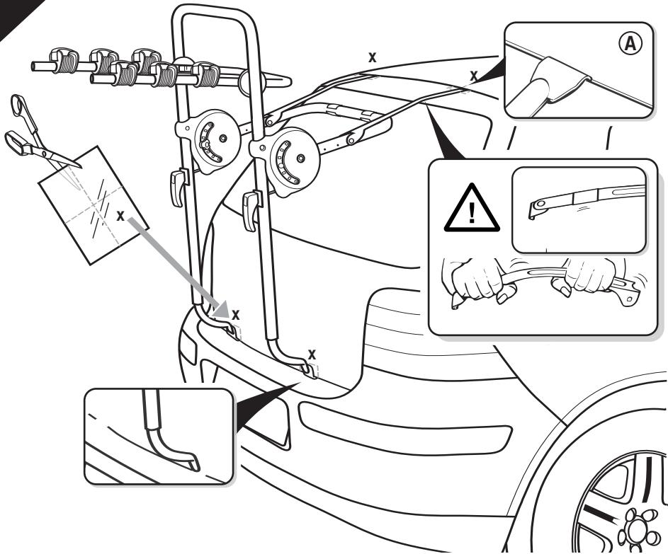
**GB.** A. Offer the carrier to the vehicle and hook the metal clamp straps over the tailgate of your vehicle.
