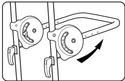
**GB.** Refer to the enclosed application list to find the correct angle for the vehicle support arm for your car. Insert the bolts from the outside faces in the specified holes A, B, C, D, E, F or G.
