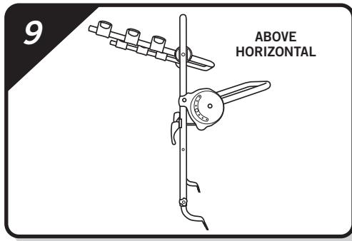
**GB.** Re-position the cycle support arm to above horizontal using the quick release handles on the ratchet adjusters.
