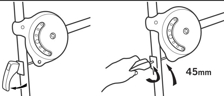
**GB.** Release the two carrier clamping levers and turn the handles anti-clockwise until the angle adjusters are fully opened, exposing approximately 45mm of the bolt.
