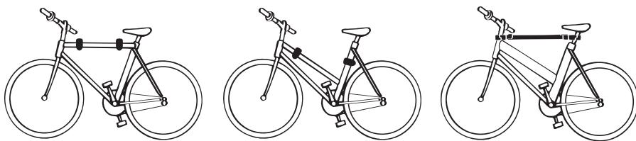
**gb.** The cycle frame locators can be adjusted to best suit the angle of ladies' and children's etc, cycle frames. A false cross bar is available, for the easy mounting of full suspension and low cross bar cycle frames.
