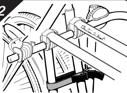
**GB.** When carrying a second or third cycle, feed the RED straps around all cycles, and fully tighten. **Failure to use these straps will result in the cycles falling off the carrier.** To reduce obstruction from the handle bars alternate the direction of each cycle during loading.
