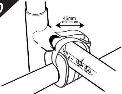
**GB.** Position your cycle(s) into the saddle area of the frame locator. Pass the webbing strap over the frame of the cycle and thread through the metal loop. Pull the strap back tightly and press the hook and loop fastener to secure.
