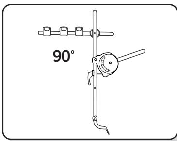
**GB.** Position the assembled carrier on a clean surface as illustrated. Release the 2 adjuster levers and rotate the cycle support arms through 90° and lock in position. The quick release action should be firm for both opening and closing. The tension may be set by releasing the handles and turning clockwise.
