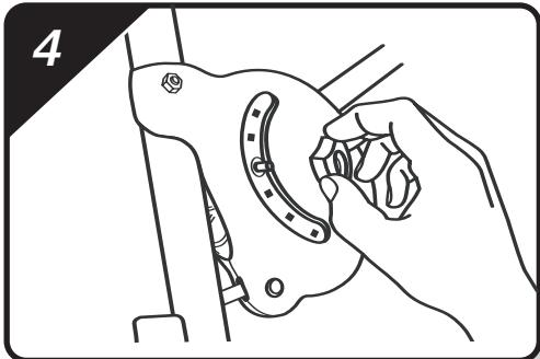
**GB.** Fit the thumb screw nuts to the inside face of the angle adjusters.
