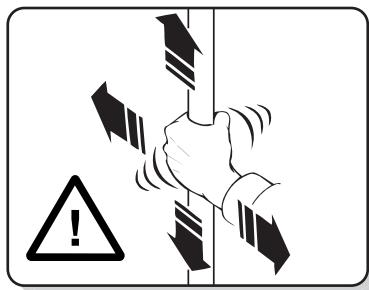
**GB.** Ensure that both carrier clamping levers are in the clamped position. Progressively tighten the levers on both sides of the carrier, by turning them clockwise. When the resistance to turning starts to increase check the security of the carrier. Continue gradually tightening both levers until the carrier is firmly fixed in all directions.
