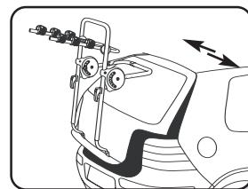
**GB.** When removing the carrier from your vehicle release both carrier clamping levers. Unhook the feet first from your tailgate (1st) and then metal fitting kit clamps (2nd). If you are experiencing difficulty in removing the carrier try opening the tailgate and sliding the metal clamps towards the outer edges of the top of the hatch.
